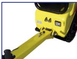
Hydraulic pump built-in the arm
