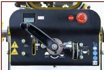
Advanced control panel with hour meter and cutting depth indicator gauge.
