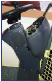
Adjustable ergonomic steering wheel
