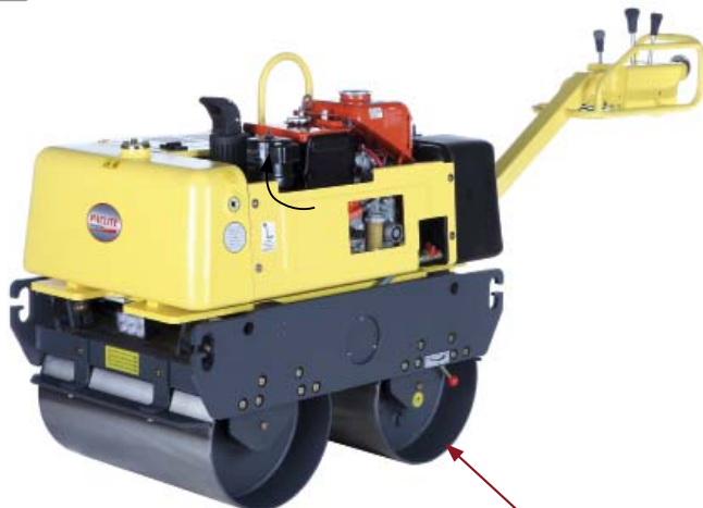
Hydraulic drive motors on each drum
