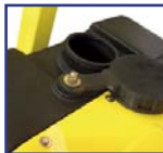
Improved water tank 47 litres
