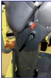
Adjustable ergonomic steering wheel
