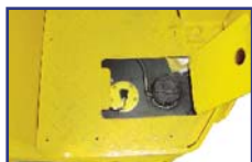
Diesel fuel cap easy access on operator floor
