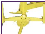
Directional and oscillating supplementary axle
